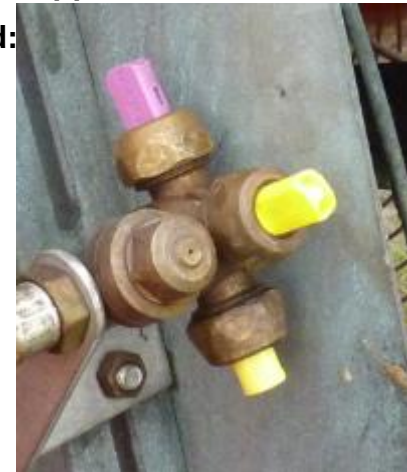
3 fold nozzle holder for quick nozzle change
